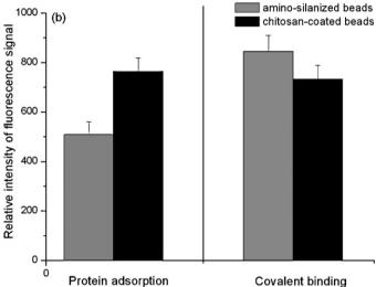
**Fig. 2.** Detection of immobilized DL488 anti-rabbit IgG on chitosan-coated beads. (a) Fluorescence signal as a function of chitosan solution concentration for DL488 anti-rabbit IgG immobilization: (circles) aldehyde-silane beads; (squares) chitosan-coated beads. (b) Adsorption or binding of DL488 anti-rabbit IgG on beads. Non-activated beads (left) and activated beads by glutaraldehyde (right). Chitosan concentration: 0.1%.
