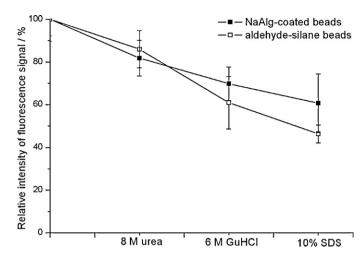
Fig. 6. Fluorescence signal of beads with varying denaturing conditions.
