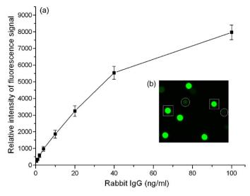
**Fig. 5.** Quantitative sandwich assays: (a) diagram of the fluorescence intensity as a function of rabbit IgG concentration in the sandwich immune fluorescence assay; (b) fluorescence microscope images of the mixed NaAlg-coated beads (goat antirabbit IgG-immobilized beads are identified by squares; BSA-immobilized beads are circled). Only goat anti-rabbit IgG-bound beads could be observed in the strong fluorescence signal.
